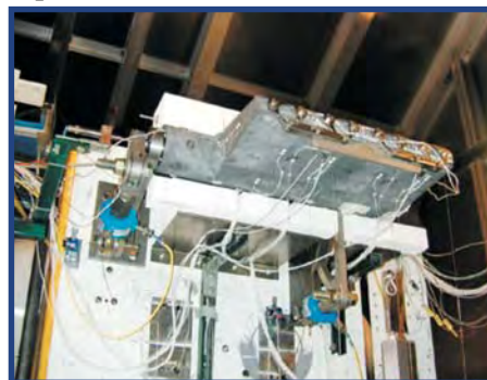
C-SiC flapperon subcomponent installed in the test setup at DFRC
